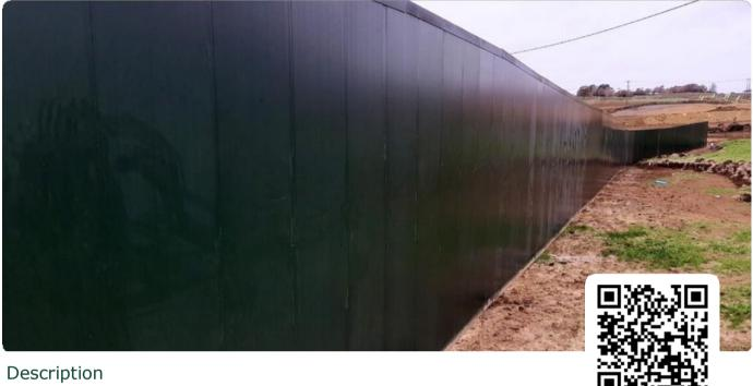
HoardSafe is CLD's range of sustainable and secure hoarding. Manufactured from composite recycled plastic panels which click easily into place and are installed on steel rails. HoardSafe S1 is a security rated version which incorporates a Securus steel mesh panel to the rear which has been certified by the Loss Prevention Certification Board to provide a minimum of 60 seconds against attack. The system can be fixed to blocks or ground buried. transportation and installation.
